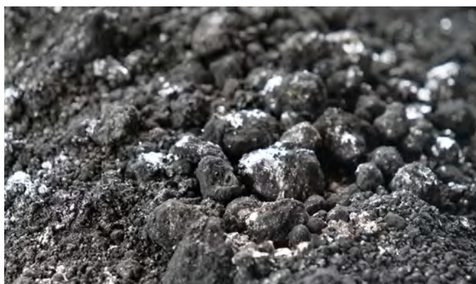
Copper-lead matte, consisting of copper, lead, sulfur and precious metals, is one of the intermediate products.
