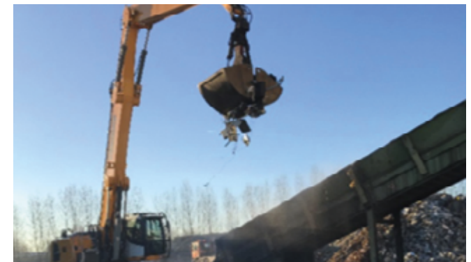
Releasing the electrical and electronic devices onto the feed conveyor of the MV-ZS facility
