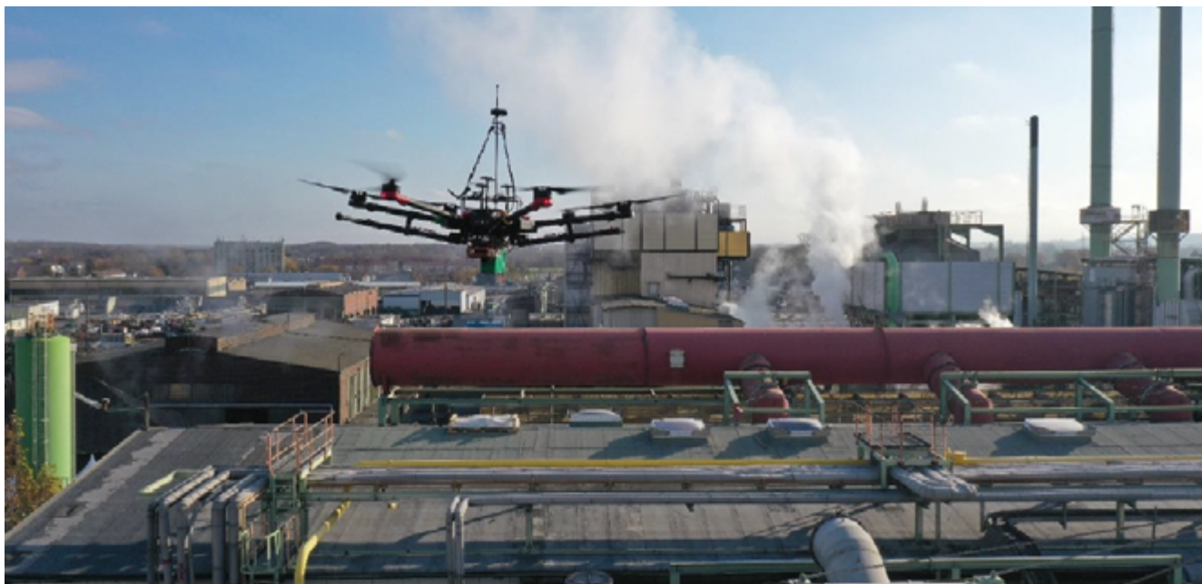
Emission measurements using drones at the Lünen plant
